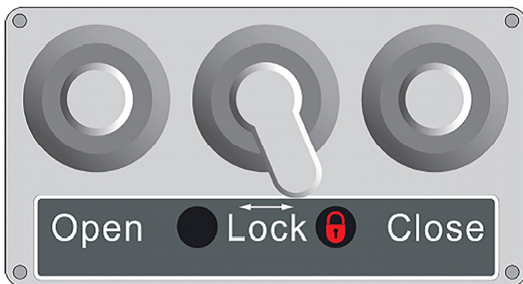
Figure M.3 — Example of door lock providing visual and tactile indication of status
