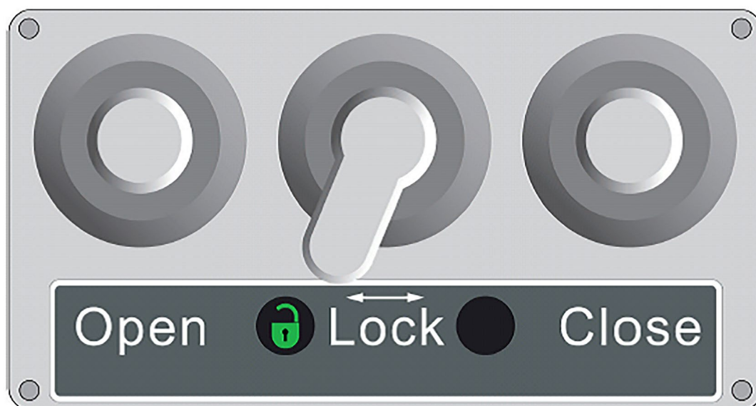
Figure M.2 — Example of door lock that provides visual and tactile indication of status
